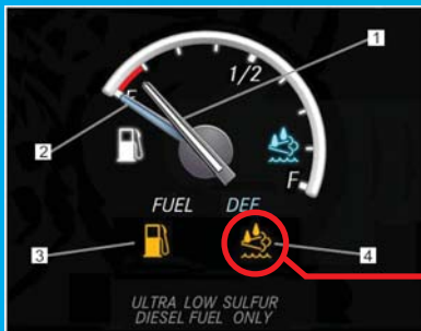
Fuel/DEF Gauge Diesel fuel and DEF levels are measured in a dual-purpose gauge.
