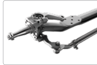
Up to a 55-degree wheel cut for added maneuverability (45-degree on Model 5).
